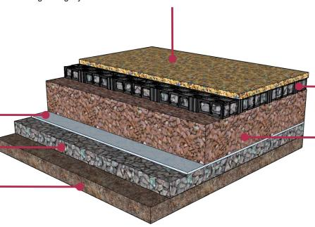
**SureCell** (Installed by SureSet or others) 52mm depth fully connected cellular reinforcement structure infilled with well compacted 4/10mm graded crushed aggregate to BS EN12620
